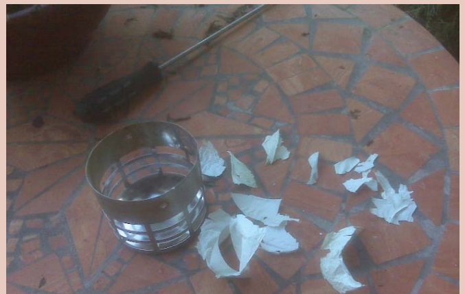
This flue pipe was discovered by a Registered Gas Installer on a boiler which showed signs of flame lift. This is the inner combustion tube taken from the boiler. The result of condense forming in the flue and attacking the metal (this is a non-condensing boiler) Its imperative that the correct fall as specified by the manufacturers is achieved on flue runs.
