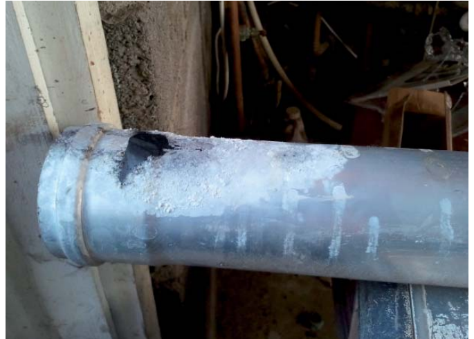
This flue pipe was discovered by a Registered Gas Installer on a boiler which showed signs of flame lift. This is the inner combustion tube taken from the boiler. The result of condense forming in the flue and attacking the metal (this is a non-condensing boiler) Its imperative that the correct fall as specified by the manufacturers is achieved on flue runs.
