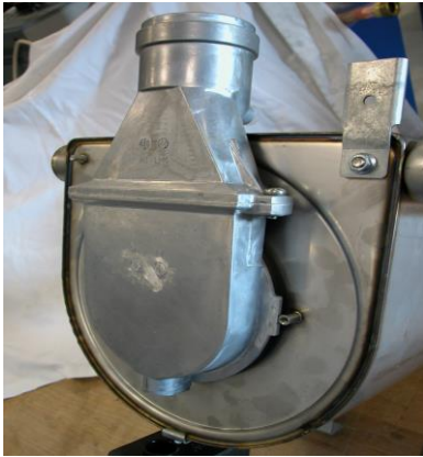
Figure 2 Aluminium flue/condensate connector attached to the rear of the heat exchanger (Photograph shows the view from the rear of the boiler)
