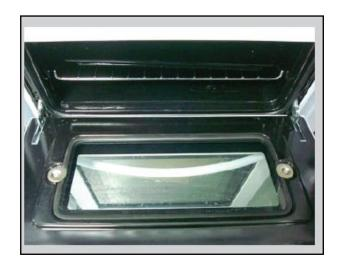
Pull the bottom of the seal away from the cooker without removing the hooks from the hole and cut the seal 35mm in from the hook on both the bottom left hand and right hand corners of the seal as shown in the picture below and remove the bottom piece of the seal.
